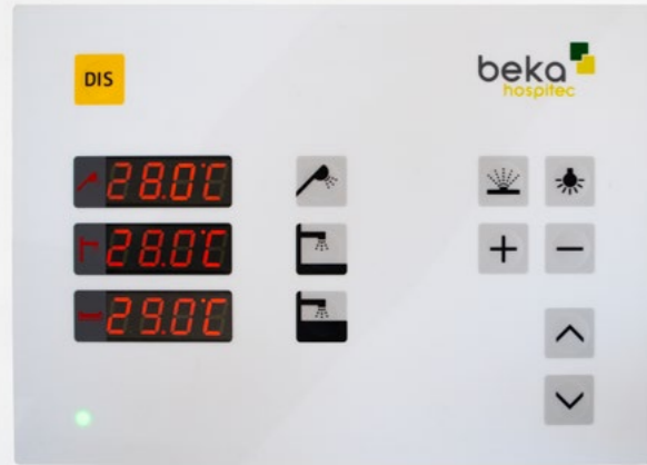
Operating panel with temperature display
